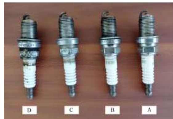
Figure 1 : View of the spark plugs used for the test with the following performance (thousands of kilometers): A) Zero to 10 B) 10 to 20 C) 20 to 30 D) 30 to 40
