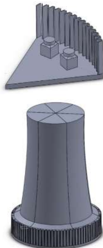
Figure 1: Geometric model of the tower and a tower sector with two peak coolers
