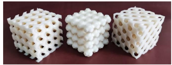
Figure 4: Printed structures; Schwarz G, P and D from left to right respectively
