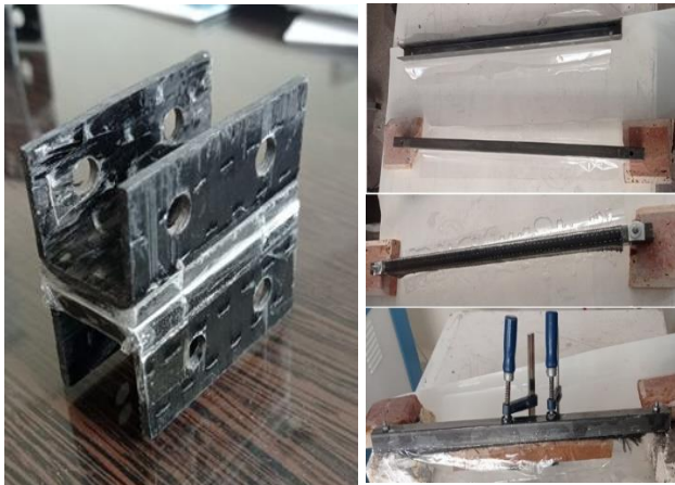
Figure 2: Steps in producing U-shaped adhesives
