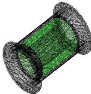
Fig. 2 The meshing of the main stator and shell model
